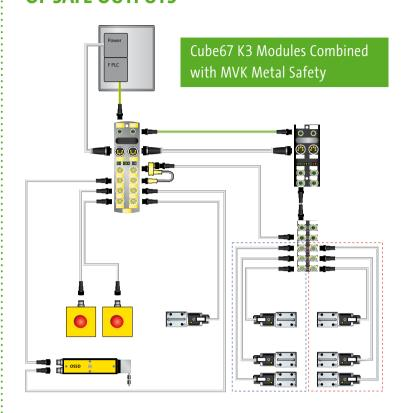
Safety technology is a major topic in the automation industry: Excellent protection for man and machine is the highest priority. Now it's possible to easily increase in the number of safe outputs within a system by using Murrelektronik's combined solution: the modular Cube67 fieldbus system and the safe fieldbus module MVK Metal Safety. This saves space in the cabinet, because safety relays are no longer necessary.
