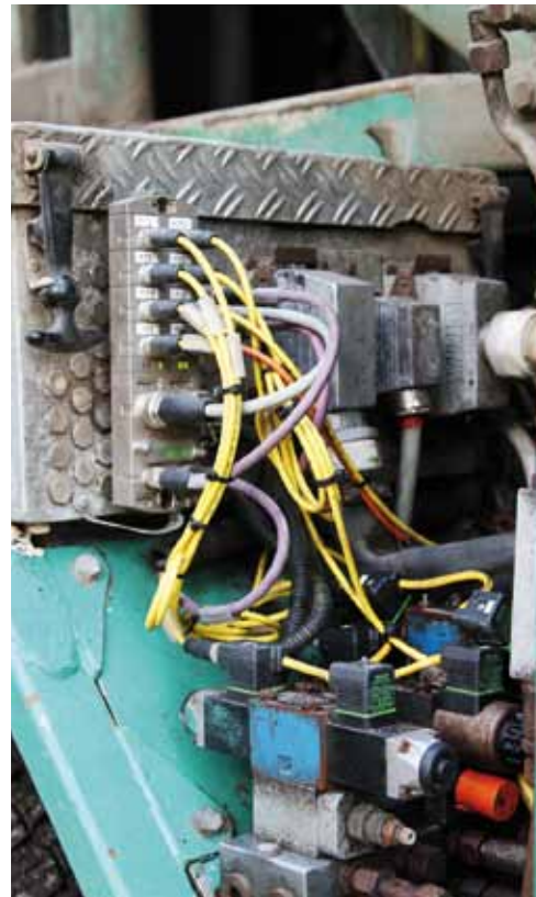
MVK Metal Close to the Process, with Double Valve Connectors
